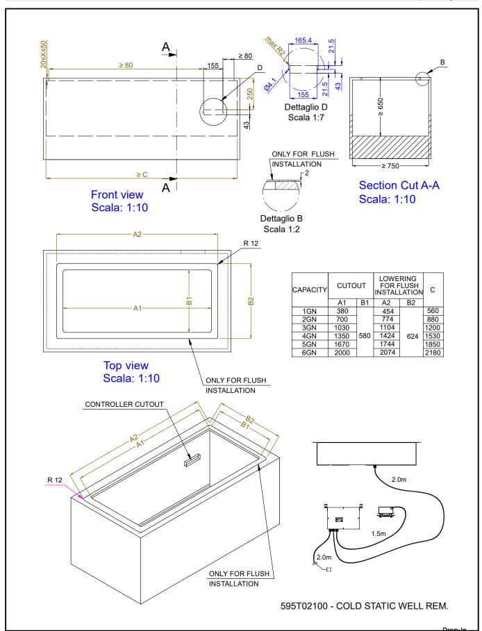
Drop-in remote refrigerated well, static (6 GN container capacity)
